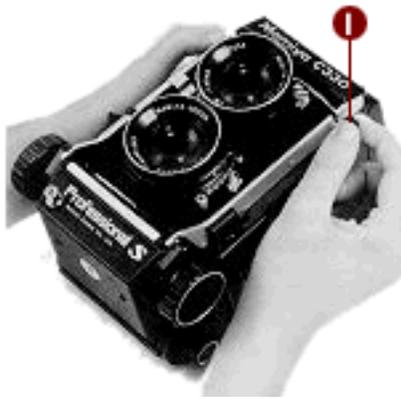
Place the camera so that the lens mount faces upward and pinch the lens clamp bracket (1), press the head toward the camera body, and move it along the groove to release the lens clamp. Now the body cap and/or lens can be removed.
