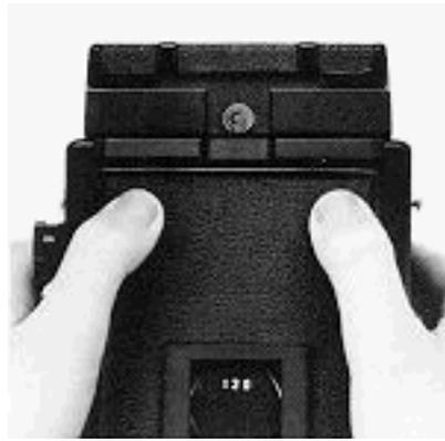
When closing the back cover, firmly press both sides of the back cover, making sure that neither side of the back cover is open or loose. Unless the back cover is closed tightly, the automatic film stopper will not work.
