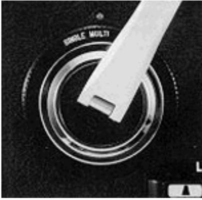
Turn the multiple exposure dial (28) and set the word 'MULTI' to the red dot, then the double exposure prevention is disengaged. The shutter button can be depressed without advancing the film, whenever the shutter is cocked manually.
