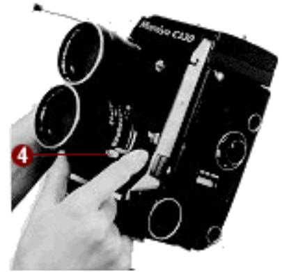
Insert the lens into the lens mount so that the lens shutter cocking lever (4) connects with the cocking lever on the camera body. This operation is more easily performed by cocking the lens shutter with the fingers and inserting the lens from the cocking lever side on the body.
