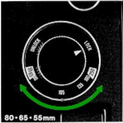
After changing a lens, set the parallax correcting dial (10) to the focal length value of the mounted lens. For 55mm and 65mm lenses, set the parallax correcting dial to 80, then attach the parallax correction plate for 55mm/65mm lenses to the focusing hood. (Refer to p.22). For the 250mm lens, set the parallax correcting dial to 180.
